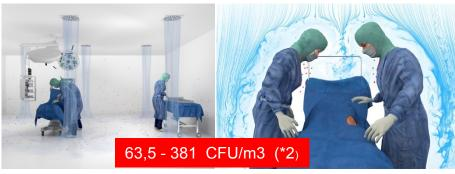
Focused laminar flow systems: the air is through hepa filters filtered free microorganisms and then directed immediately onto the surgical instruments and surgical site. It is only then distributed throughout the operating theatre. This protects the critical area of the operating theatre, i.e. the instruments and the surgical site. With this system, the bacterial load on the instruments and surgical site is reduced by than 95% compared conventional ventilation systems.
